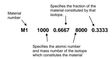
In this example, the material is water, which is made of 0.6667 parts hydrogen, to 0.3333 parts oxygen. Hydrogen is represented as 1000. The 1 refers to an atomic number of 1 and the remaining 3 digits relate to the isotope. In this case, however, because the example uses photon transport only, the isotope number does not have to be given. If no numbers are specified for the mass number, MCNP will assume the natural abundance of that element.
