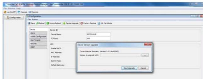
2. The current IP firmware version will be displayed in the center of this screen. Compare the current version with the version on Tripp Lite's website to determine if you need to upgrade your KVM.
