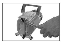
→ Use an open end wrench (width 15mm) to assemble the screw-in fitting with connection hose to the pump head. If necessary, steady with an open end wrench (width 16mm).
