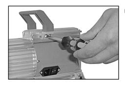
→ Loosen the two screws (use Phillips screw driver) at the handle and remove handle.
