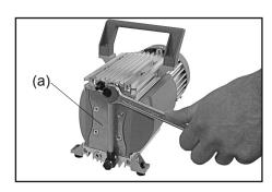
→ Use an open end wrench (width 15 mm) to remove the screw-in fitting from the pump head, and remove along with the connecting hose.
