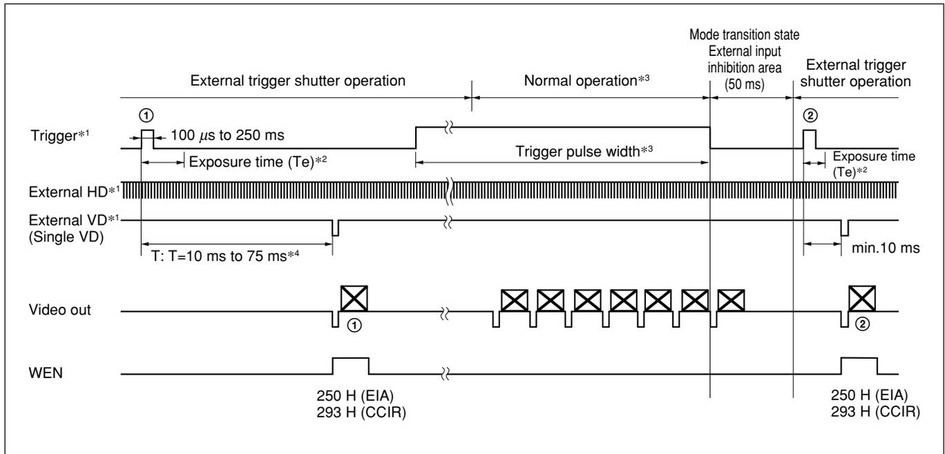
\*1 This is a signal input from outside. Make sure to input both HD and VD signals in this case. Input the signal so that the VD phase aligns with the HD falling edge.
