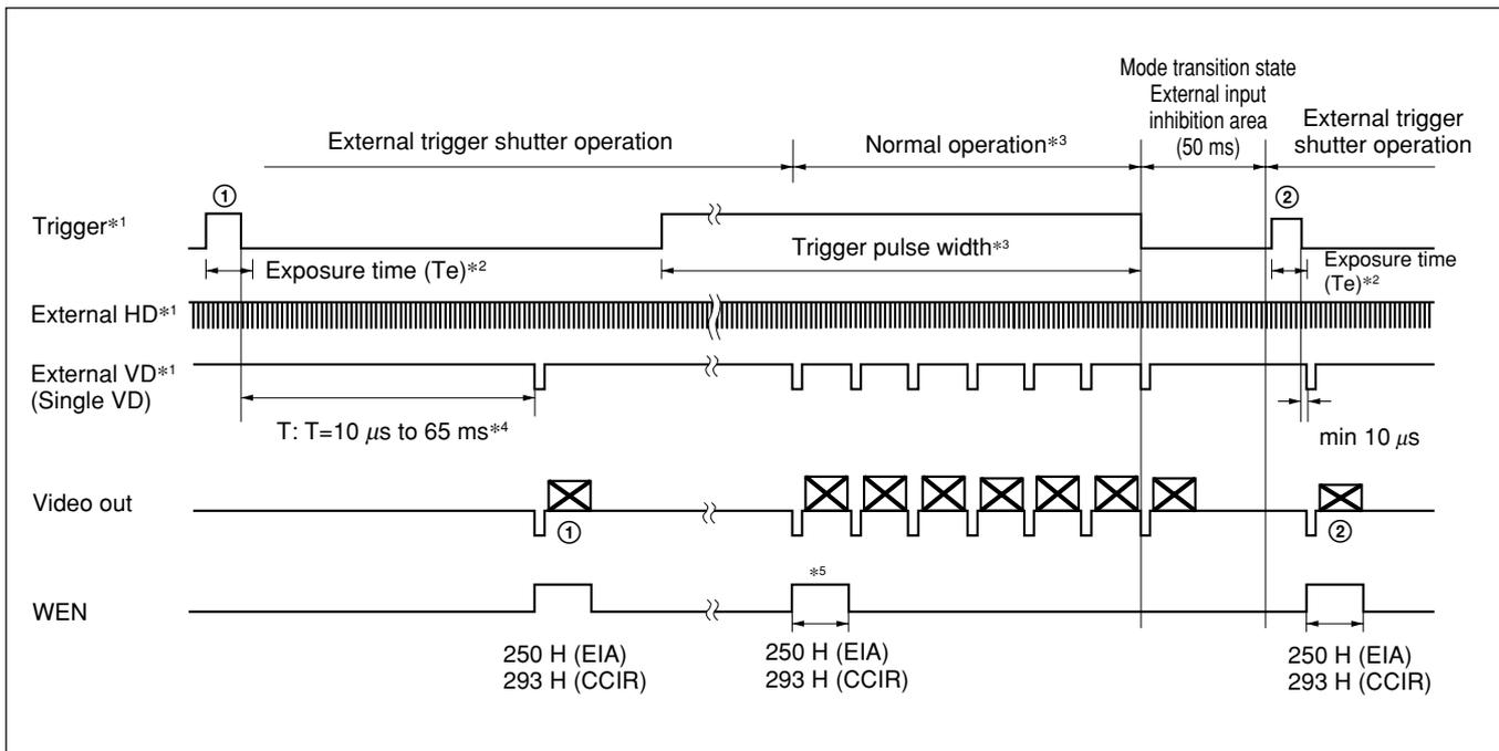
\*1 This is a signal input from outside. Make sure to input both HD and VD signals in this case. Input the signal so that the VD phase aligns with the HD falling edge.
