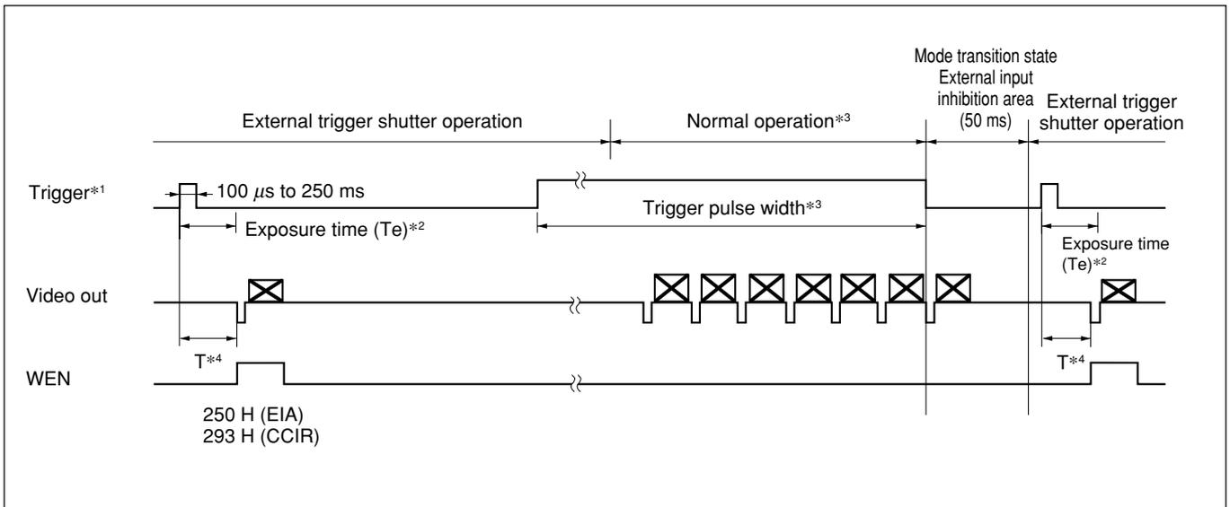
\*1 This is a signal input from outside. The trigger input frequency must be [Shutter speed (DIP switches) + 1 field + 2 H frequency] or more. If invalid data is input, normal operation is resumed several Vs after entering the correct data.
