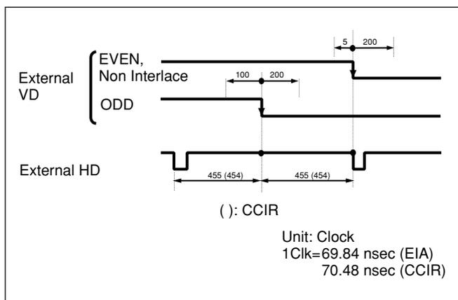
Make sure that the external HD/VD phases against the standard central phase are as shown in the figure above. Invalid signal input may cause an error in the internal reset.
