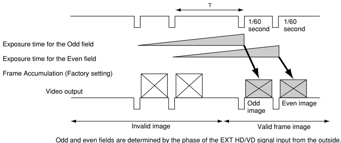
Odd and even fields are determined by the phase of the EXT HD/VD signal input from the outside.
