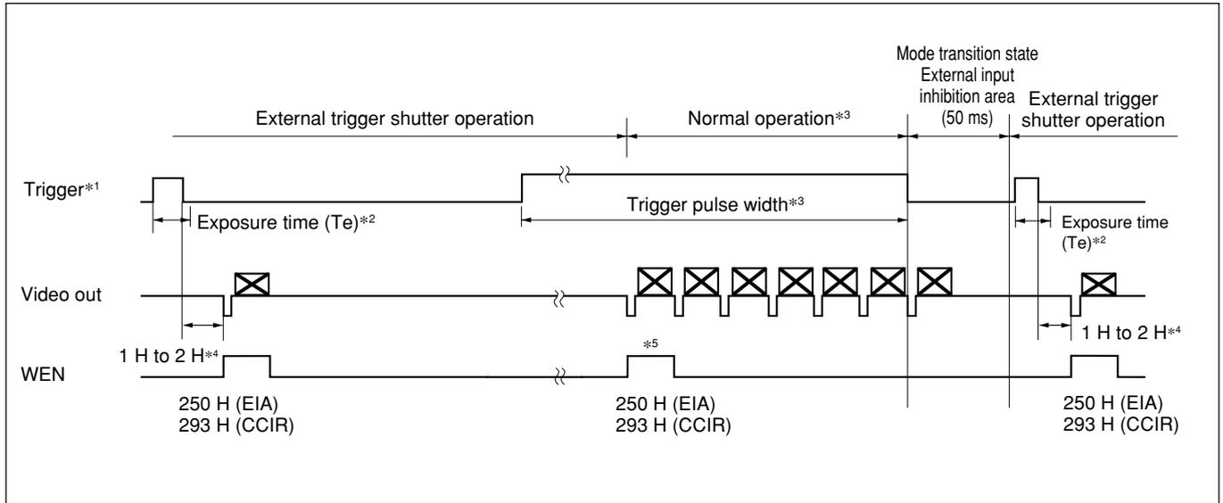
\*1 This is a signal input from outside. The trigger input frequency must be [Trigger pulse width + 1 field + 2 H frequency] or more. The operation is not guaranteed for shorter frequencies. If invalid data is input, normal operation is resumed several Vs after entering the correct data.
