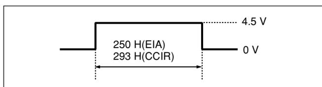
The amplitude level is the typical value when terminated with 10 kΩ.
