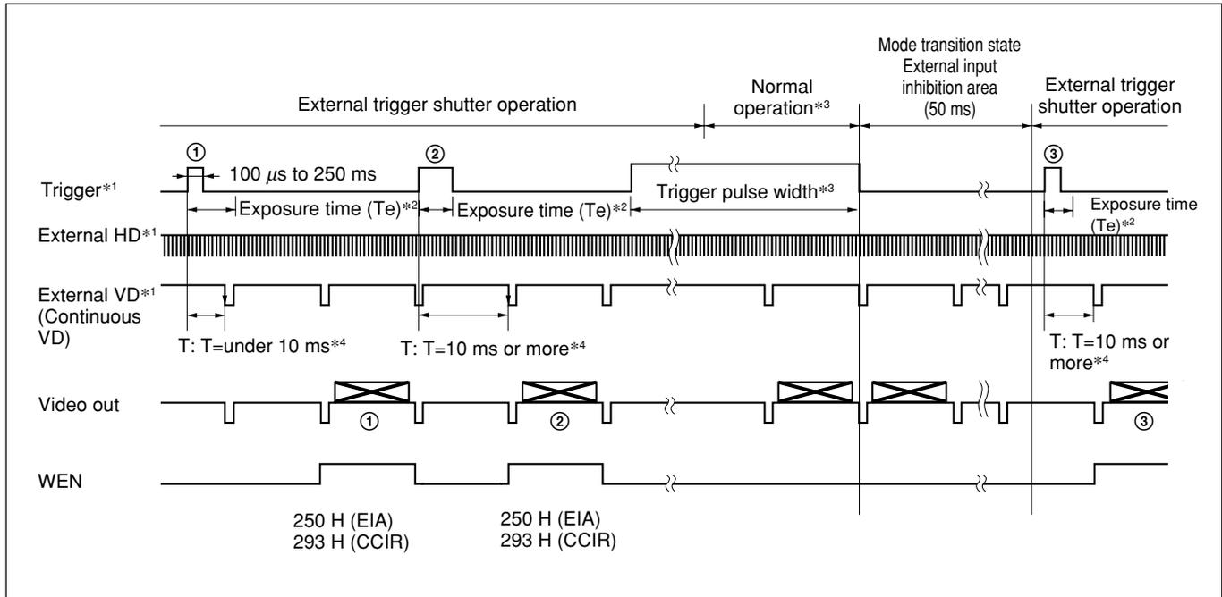
\*1 This is a signal input from outside. The continuous VD frequency is one field. Make sure you input HD and VD at the same time.
