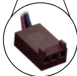
Close-up of fan connector
