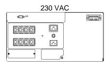
Notes: The larger 120 VAC units (1400RMXL, 2200RM, 3000RM, 2200RMXL) require a 20, 30, or 50 amp plug. These plugs require a special outlet to be installed by a certified electrician. The rear panel of a 3000RM (5U) will support one SU48BP additional battery pack; the 3000RM (3U) does not.
